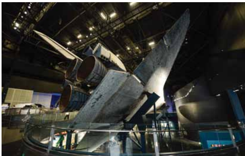
View from behind showing vast underside and heat tiles
